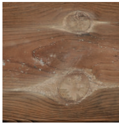
Round knots/Nudos redondos/ Noeuds ronds/Runde knoten / Nodi rotondi/ Ronde kwasten/ Nós redondos
