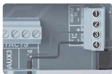
Free Chlorine probe ③ red ④ black
