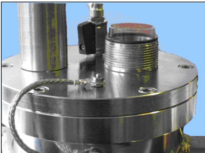
Insert the o-ring on the sleeve (point 8)
